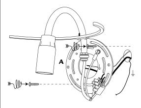
4. Place the metal plate **B** over the element **A**. Then screw the screw **C** and install bulb. Do not exceed the maximum wattage for this fixture. Refer to the wattage warning label attached to the fixture for maximum allowable wattage.
