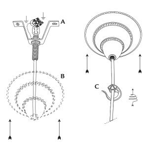
5. Screw the hook **C** onto the nipple and tighten securely.
