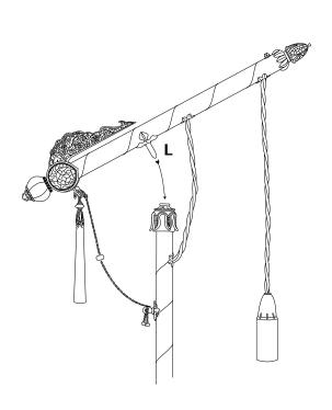
5. Place the rod in horizontal position inserting the peg L into the stand.
