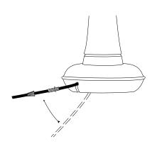
2. Insert the wooden cone into the base.
