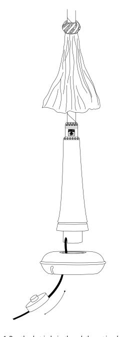
1. Pass the electrical wire through the cast iron base.
