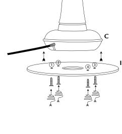
4. Fix the metal disk I to the base C with the 4 screws.
