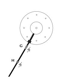
3. linsert the wire within the groove and fix it to the base with elements G and H.
